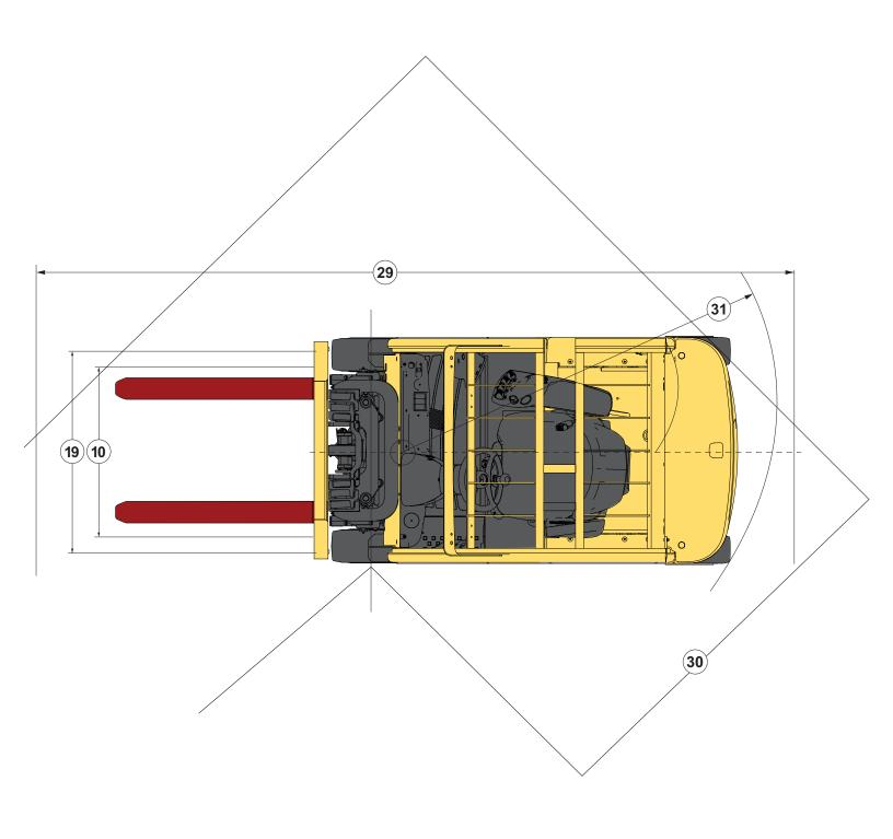
Circled dimensions correspond to the line numbers on the tabulated chart inside the technical guide. Dimensions are in inches (millimeters).
