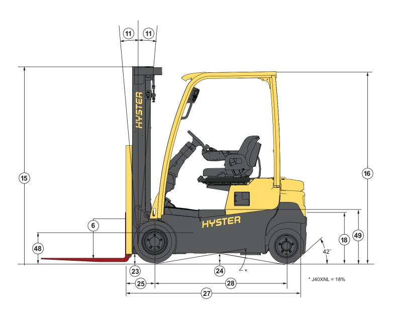
Circled dimensions correspond to the line numbers on the tabulated chart inside the technical guide. Dimensions are in inches (millimeters).
